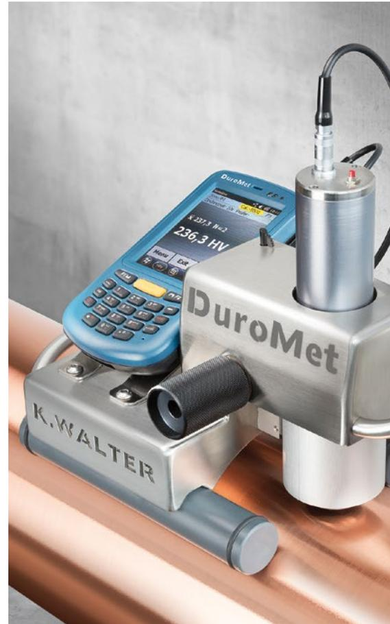
DuroMet: Test probe with Vickers diamond
